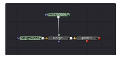
The distinction if an Input or Output is on the flow is made by defining them as MainInput and MainOutput during the development of the Plugin or Fuse.
